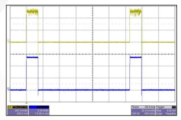
Figure 18: A short circuit across the output terminals. Ch 1: Vout (200mV/div). Ch 2: Iout (5A/div).
