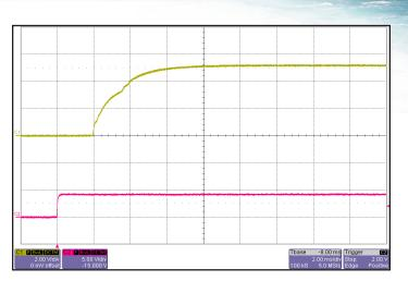
*Figure 8:* Turn-on transient at full resistive load and zero output capacitance initiated by On/Off. Input voltage pre-applied. Ch 1: Vout (2V/div). Ch 2: On/Off (5V/div).
