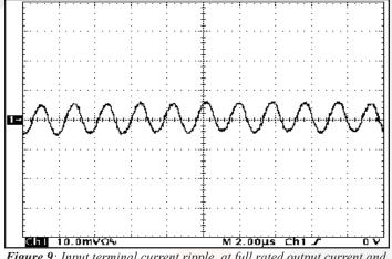
*Figure 9*: Input terminal current ripple, at full rated output current and nominal input voltage with SynQor MCOTS filter module(20mA/div.) See Figure 17.
