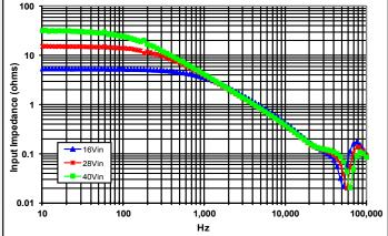
**Figure 16**: Magnitude of incremental input impedance  $(Z_{in} = v_{in}/i_{in})$  for minimum, nominal, and maximum input voltage at full rated power.
