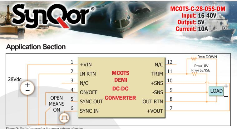
Figure D: Typical connection for output voltage trimming.
