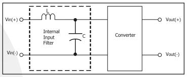
Figure F: Internal Input Filter Diagram.
